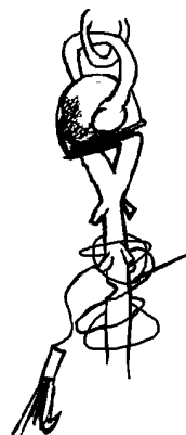
Partially cut mooring rope
