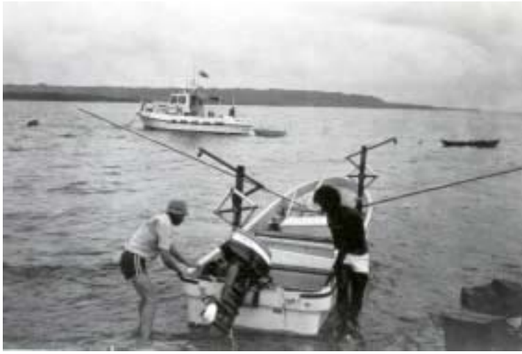
Fibreglass trolling booms rigged on a small Japanese skiff
