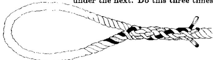
To make a tapered splice, make additional tucks with two of the ends so that all three finish at different places, then cut off.
