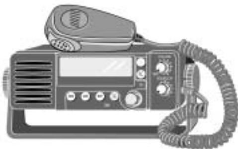
**VHF — very high frequency radio:** provides short range radio communications, essential for communicating with harbour authorities, with agents, and with other vessels in crossing situations to avoid collisions.
