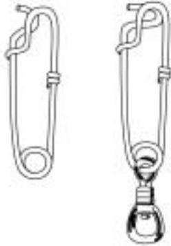
The swivel snap — often called a clip — is a very important component of a branchline. There are different snaps for rope and monofilament gear, and they should not be interchanged, as they will not work properly. Snaps made for rope gear have a jaw that is too big to grip monofilament mainline. The branchlines will slide freely and cause tangles. Conversely, the jaw of a snap for monofilament gear is too small to work properly on the larger diameter rope gear.
