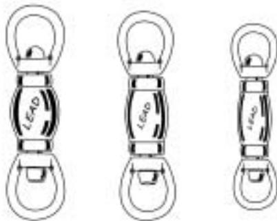
Other swivels can be used in the construction of branchlines, although they do not have the weight of the leaded swivel. Box and BL swivels can be used on rope gear, both in the mainline and in the construction of branchlines. For monofilament branchlines, crane or torpedo swivels can be used.
