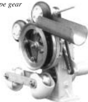
A line setter cannot be used on rope gear where the branchlines are left attached to the mainline, or where the mainline is stored in disconnected section. In these cases, coils of mainline are thrown by hand in such a way that the line is going out at a rate faster than the boat is travelling.
