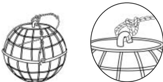
A good way to attach the short line to the float is to run the eye splice through the ear, double the eye over, then run the end with the snap through the double loop. The result is a knot that will tighten up on the standing part of the rope and will not move on the ear of the float. This knot will not chaff through.
