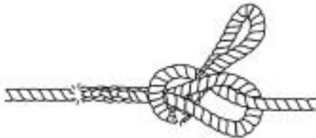
Branchlines are usually spaced about 50 m apart on the mainline, and are attached to specific joints made with two eye splices, using a sheet bend. Floatlines with floats are attached between the baskets, also on joints.
