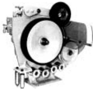
*Line setter for rope gear*
