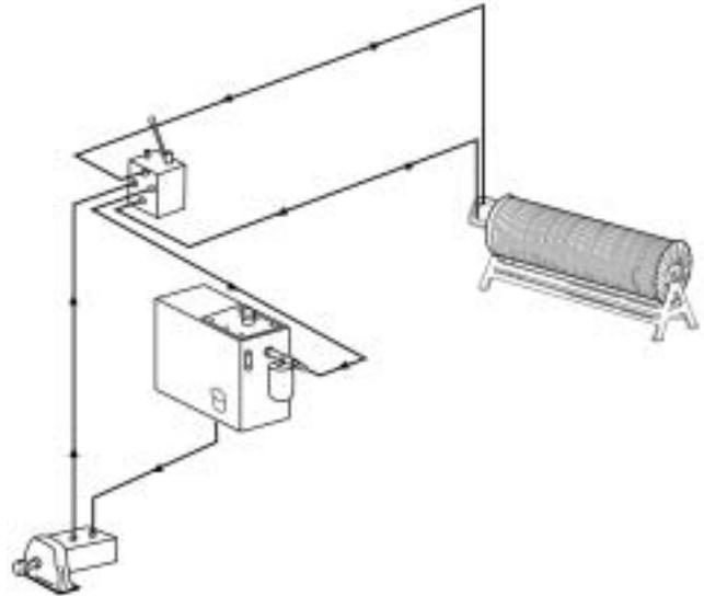
Hydraulic systems are rated by volume and pressure of fluid available for work. A typical longline system requires 15 gallons per minute (GPM) at 1200 PSI. The important thing is that the ratings of the pump match the requirements of the hydraulic motors or rams.
