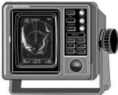
**Radar:** is essential for safe navigation, especially in areas where there are abundant reefs or where there may be other vessels. If fishing is done within radar range of shore, radar can be used to plot positions of a longline set. A radar unit with a 24 nm range should be sufficient for a small-scale longline vessel, while 36 nm range should be sufficient for a medium-scale longline vessel.
