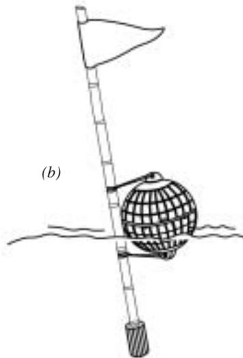
The second method is to have the flagpole separate from the float, just attached to it. In this case, the pole is weighted on the bottom and a flag placed on the top. A short piece of tarred line is attached to the pole so that it can be attached to the float either by a snap or a sheet bend. The pole sits beside the float in the water with the weight keeping the pole upright (c). This allows the flagpoles to be stored separately, plus it allows the floats to be used for other purposes as well.
