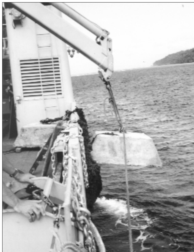
Figure 12: Mooring line flaked on back deck with ends going over the stern through a fairlead
