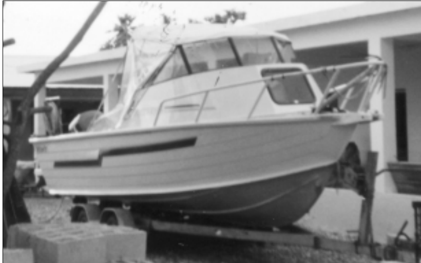
Figure 8: The 7 m aluminium 'Yellowfin' design boat used for the Futuna site survey
